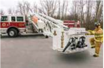
Basket accessible from ground at full retraction
