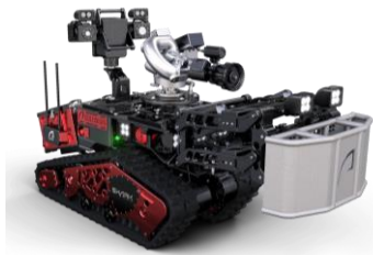
COLOSSUS FIREFIGHTING MODULE Water canon + Video turret + motorized bull bar
