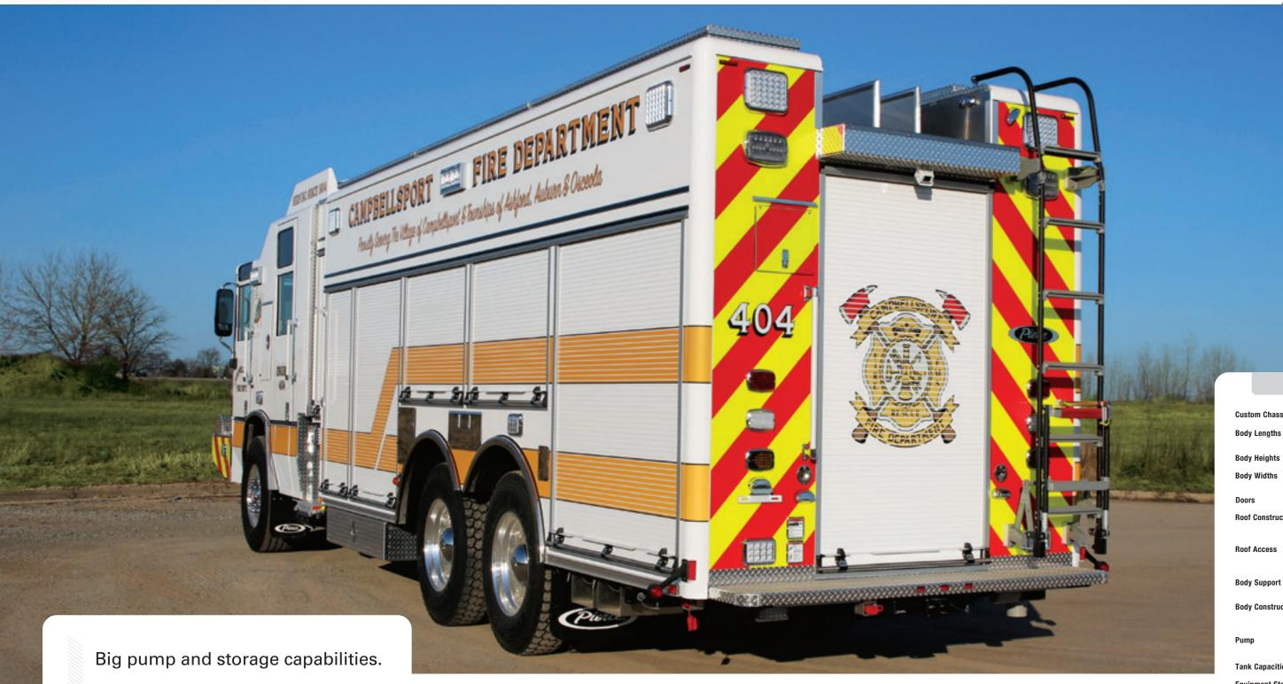
PUC™ heavy-duty rescues minimize space used for fire suppression to maximize storage options – while still delivering 1,500 gpm with a single-stage pump.
